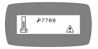
**3. 770, 7701, 7702, and 7703 ERROR:** The vacuum motor has exceeded their authorized power limits. Turn *OFF* Key and turn *ON* again to clear.
