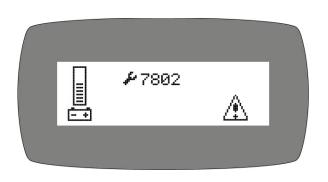
**8. 7802 ERROR:** The traction motor pulled excessive current perhaps running a ramp for more than the 60 seconds allowing for this. Turn *OFF* the Key, turn on again, and continue. You should not use this machine to climb ramps so steep and so long that this code comes up repeatedly, or you could overheat the traction motor.
