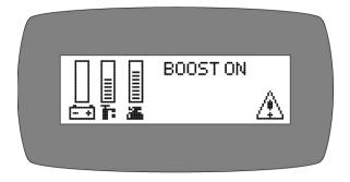
**4. BOOST ON:** Allows front wheel drive to draw more power when needed to climb ramps for 30 seconds.
