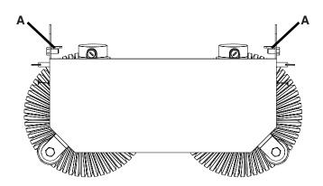
4. To move Side Broom system out of the way when not in use, just pull the pin (B) on each side of the Scrubdeck and rotate Side Broom System to the up position and reinsert pin (SEE BELOW).
