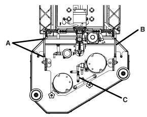
6. Extending the Adjustable Arms raise the front and lowers the rear of the Scrubdeck. After Scrubdeck has been leveled (ensure correct pitch backward - if you have) - retighten Locking Nuts (A).
