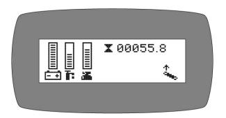
**6. Throttle ERROR:** You pressed the foot pedal before turning on the key. Turn *OFF* the key and try again, leaving foot off the pedal.
