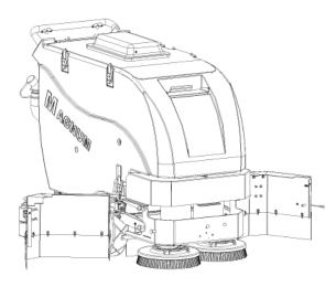
5. Tip Tank Back carefully until supported by strap (SEE BELOW).
