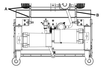
Extending the Adjustable Arms raise the front and lowers the rear of the Scrubdeck. After Scrubdeck has been leveled - retighten Locking Nuts (A).
