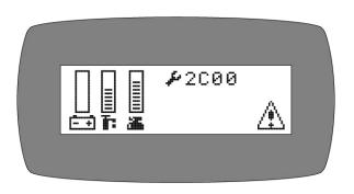
**7. 2C00 and 2C01 ERROR:** Low voltage warning. Voltage has dropped down below the minimum required to operate the machine. If you wait a few minutes, the Batteries may come up in voltage, allowing you to drive very slowly to the recharge station. If not, you will have to release the parking brake (on the front wheel, pull lever toward the front of the machine to release) and push the machine to recharging station. You must disconnect the traction motor! (+ cable first)
