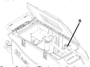
Remove Drain Hose (C) and open to allow for drainage of the Recovery Tank (SEE BELOW).
