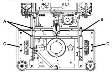
Extending the Adjustable Arms raise the front and lowers the rear of the Scrubdeck. After Scrubdeck has been leveled - tighten Locking Nuts (A).
