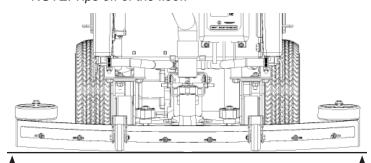
This Squeegee is adjusted too far forward and will not pick up in the center (SEE BELOW). NOTE: Center spaced off the floor.
