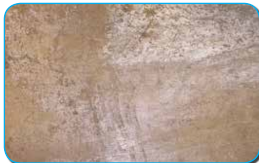
FIGURE 5-B: LEAVING DENSIFIER ON THE FLOOR TOO LONG CAN CAUSE DISCOLORIZATION.
